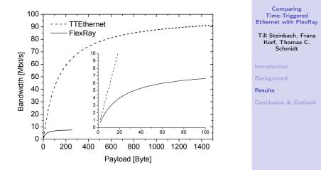
• TTEthernet allows varying payload sizes in the cycle and parallel message transmission
