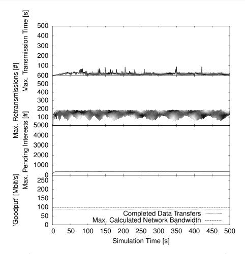
Figure 4: Simulation run; 20 Producer located at core nodes with 100 Consumers nodes at the network edge
