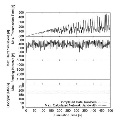
Figure 6: Simulation run; 20 Producer located at core nodes with 200 Consumers at the network edge
