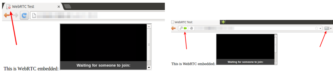
Figure 2.2: Once a WebRTC application has gained access to the camera/microphone browsers show an indicator of a call in progress so that the user knows of a possible image/sound transfer to another peer. Chrome (left) puts this indicator on the top of the tab while Firefox (right) shows it in the address bar as well as permanently right to the address bar so that even when the user is in another tab she knows of the call in progress.
