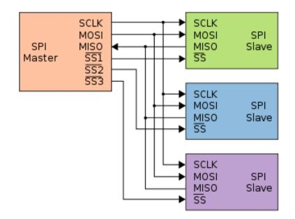
FIGURE A.2. Typical SPI bus: master and three independent slaves [7].
