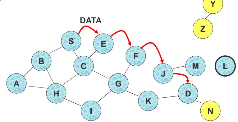
Routing table entries used to forward data packet. Route is *not* included in packet header.
