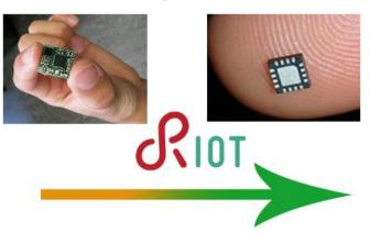
Processor: GHz, 32/64 Bit Memory: M/Gbytes Energy: Watt Network access: 5G, WLAN Processor: MHz, 8/16/32 Bit Memory: kbytes Energy: MWatt Network access: 802.15.4, BLE
