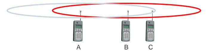
If C for example was an arbiter for sending rights, terminal B would drown out terminal A already on the physical layer Also severe problem for CDMA-networks - precise power control
