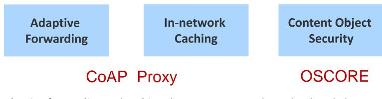
Adaptive forwarding and caching shorten request paths and reduce link traversals on retransmissions Content object security enables end-to-end security and reduces session management complexity
