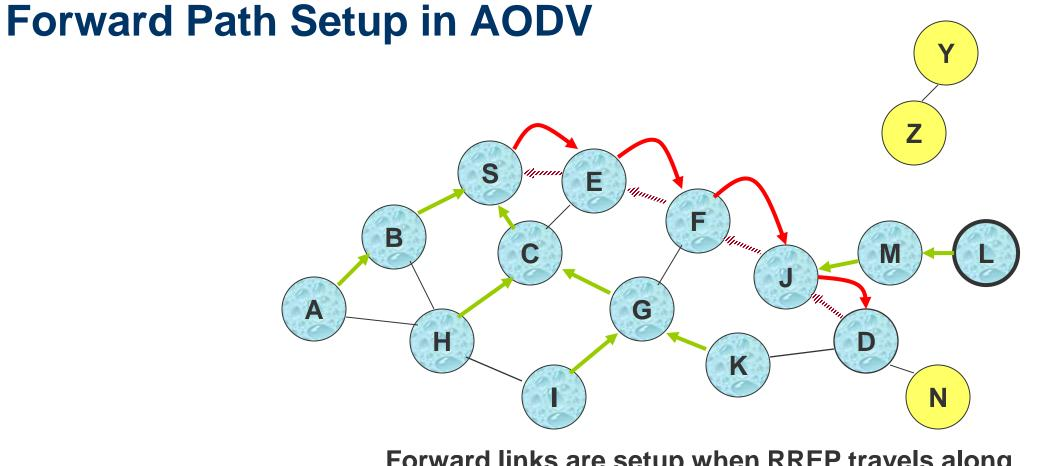
Forward links are setup when RREP travels along the reverse path
