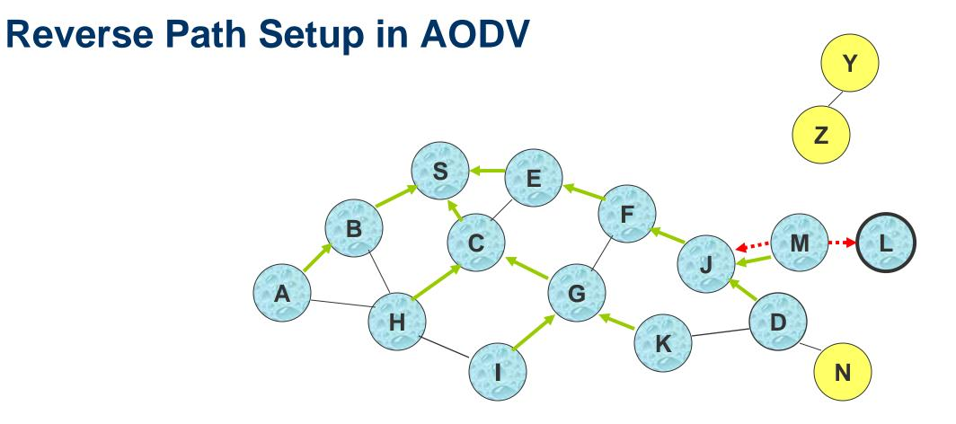
Node D does not forward RREQ, because node D is the intended target of the RREQ
