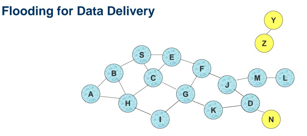
Flooding may deliver packets to too many nodes (in the worst case, all nodes reachable from sender may receive the packet)
