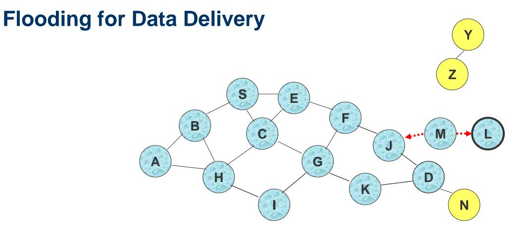
Node D does not forward packet P, because node D is the intended destination of packet P
