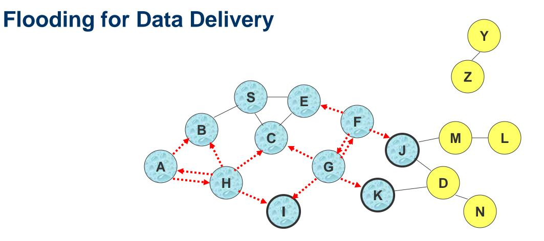
• Node C receives packet P from G and H, but does not forward it again, because node C has already forwarded packet P once
