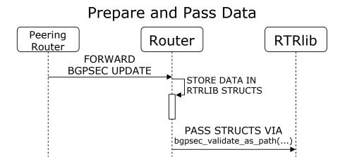
Figure 4.3: A peering router forwards a BGPsec update. The receiving router extracts the data and stores them in RTRlib structures. These structures are then passed to RTRlib.
