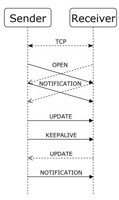
Figure 2.2: After a TCP connection is established, both routers send an open message. If they agree with the configurations, they send a keepalive message. They now send updates as they please. To keep the connection up, they send keepalive messages. Before closing the connection, a notification message is sent.
