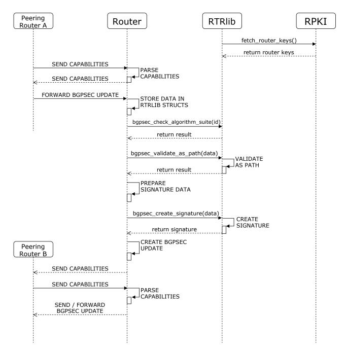
Figure 4.6: The whole workflow of processing a BGPsec update from receiving it from peer A, to forwarding it to peer B.
