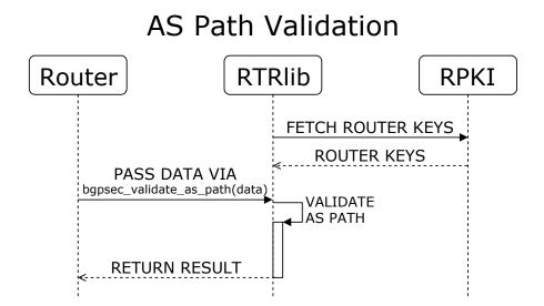
Figure 4.4: At first, RTRlib fetches all router keys from the RPKI since they are later required for the validation. When the software router passes the validation data to RTRlib, the library triggers the validation process and returns the result back to the router.
