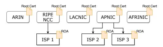
Figure 3.1: The architecture after which certificates are passed down. This structure is similar to the resource allocation hierarchy of IP prefixes.
