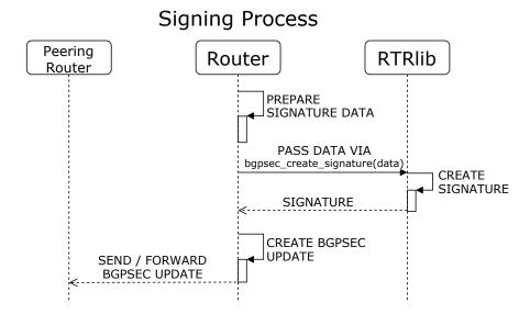
Figure 4.5: The router prepares the data that is necessary for the generation of a signature and passes it to RTRlib. The library creates and returns the signature. The process for originating a BGPsec update and forwarding an existing one is identical in this diagram.
