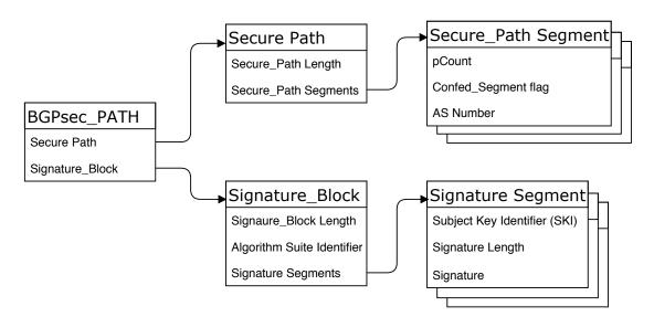
Figure 3.4: Structure of the BGPsec\_PATH attribute in an UML like fashion. Both the Secure Path as well as the Signature\_Block may contain multiple Secure\_Path Segments and Signature Segments.
