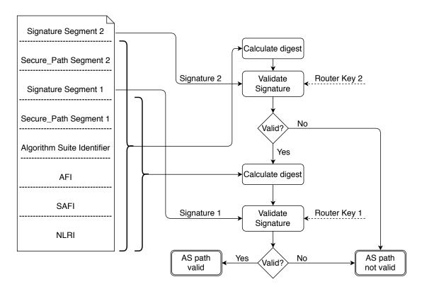
Figure 3.5: On the left is the BGPsec\_PATH attribute with the AS path (2, 1). On the right is the AS path validation process of the receiving AS 3. The process is slightly simplified for the sake of illustration.
