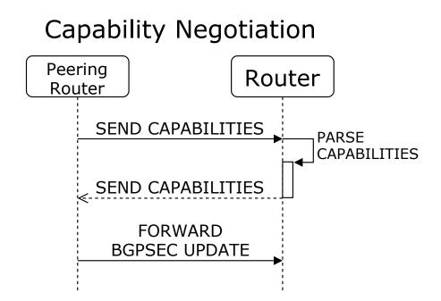
Figure 4.2: Before a router receives BGPsec updates, the capabilities must be exchanged via the open message. After a successful negotiation, BGPsec updates can be exchanged.
