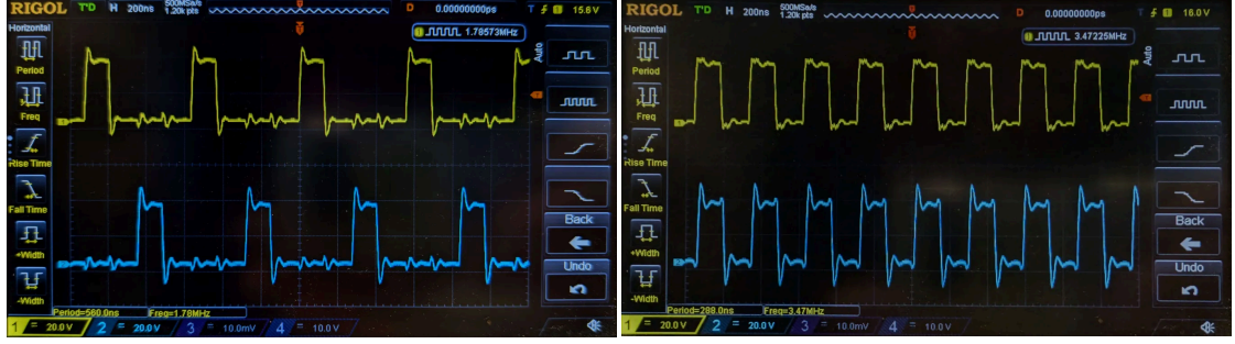
Figure 9: Oscilloscope captures showing single-core GPIO toggling (left) and dual-core GPIO toggling (right). Yellow (Top) is PIN 14, Blue (Bottom) is PIN 15. Single core average period: 560 ns, Dual core average period: 288 ns.
