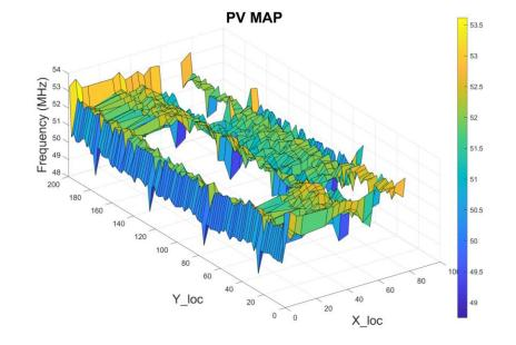
Using placement information, a frequency degradation map can be created, by measuring individual ROs
