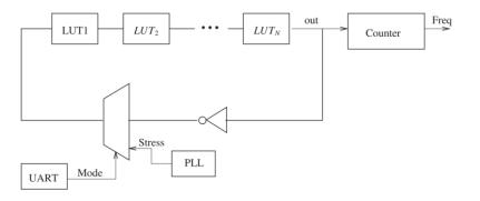
Fig. 1. RO-based sensor structure.
