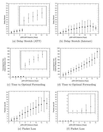
Figure 7 Performance Results for Real-World Topologies of 154 (ATT - left) and 1.540 (Internet - right) Core Nodes. Error Bars Indicate Standard Deviations
