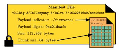
Figure 8.4: Manifest description and fixed-length chunks of a corresponding firmware image.
