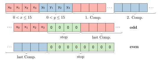
Figure 4.4: Stateless name compression and stop marker for odd and even number of name components.
