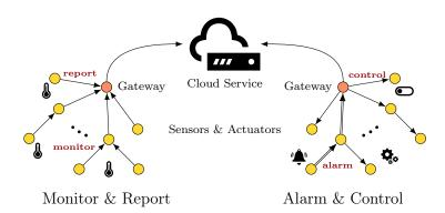
Figure 3.1: Communication flows in IIoT environments.
