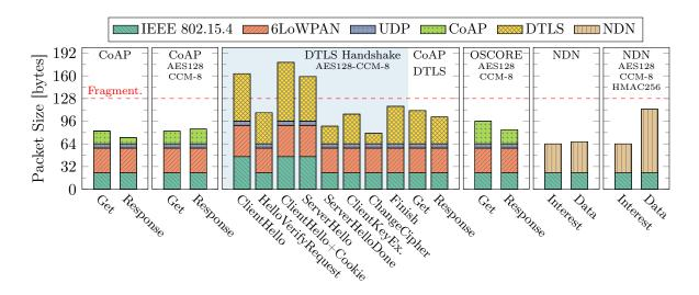
Figure 9.3: Packet structures of control- and data-plane packets for each protocol configuration.
