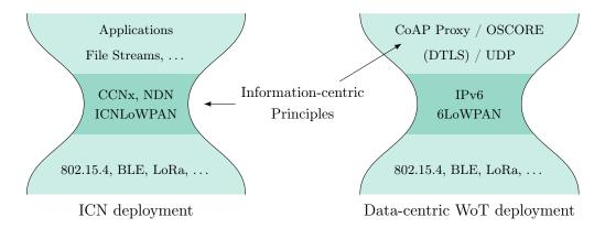
Figure 7.2: For ICN deployments, information-centric principles are located on the network layer, while they reside on the application layer for the data-centric WoT deployment.
