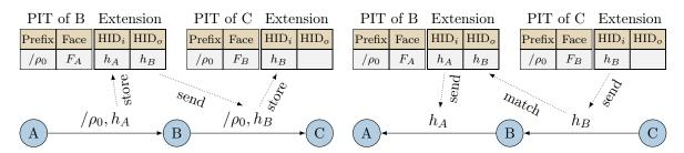
(a) Collecting compression state en-route (Interest). (b) Eliding Name TLVs using en-route state (data).
