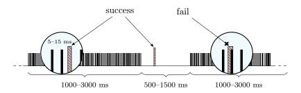
Figure 4.16: Radio interference due to bursty cross-traffic.
