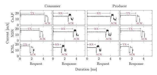
Figure 4.11: Current consumption for send and receive operations.
