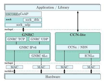
Figure 9.2: The RIOT networking subsystem.
