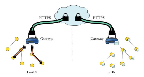
Figure 7.1: The complete deployment view for the host-centric and information-centric deployment options.
