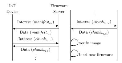
Figure 8.7: Iterative retrieval of firmware chunks.
