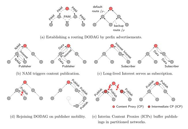
Figure 6.2: Overview on the HoPP protocol operations: topology management, publish-subscribe, mobility and delay-tolerance support.
