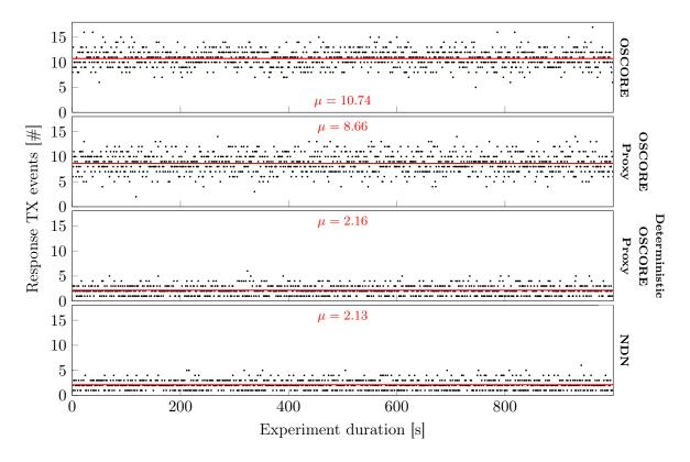
Figure 11.8: Quantity of outgoing responses measured at the server node.
