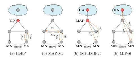
Figure 6.10: Topology setup and mobility-related signaling for the selected protocol ensemble.
