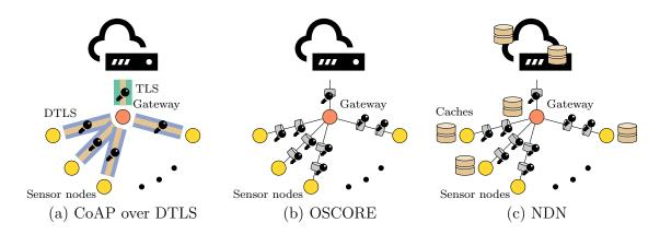
Figure 9.1: Typical deployment setups for CoAP over DTLS, OSCORE, and NDN in the IoT. Validity of session keys terminates at gateways for transport layer security due to transport conversions, e.g., UDP to TCP. Content object security is unaffected by gateway operations and reaches end-to-end.
