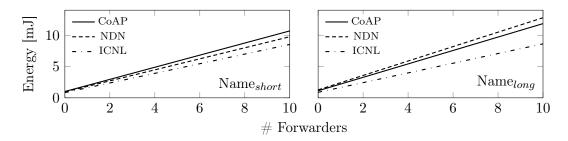
Figure 4.12: Total energy consumption for multi-hop networks.
