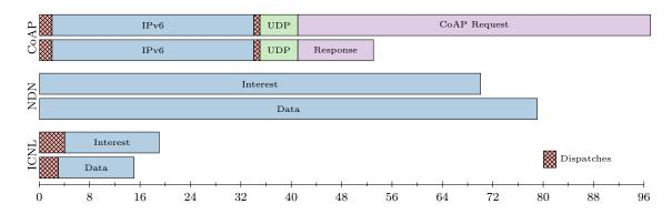
Figure 4.7: Packet length and structure for different protocols.
