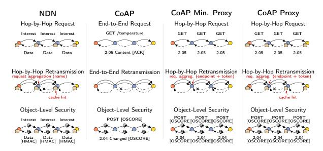
Figure 10.1: Deployment scenarios and protocol configurations used in our comparative evaluations.
