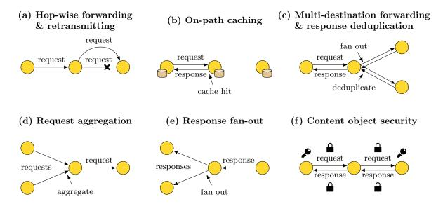
Figure 11.2: NDN protocol features that enable an efficient and secure multiparty communication for the IoT.
