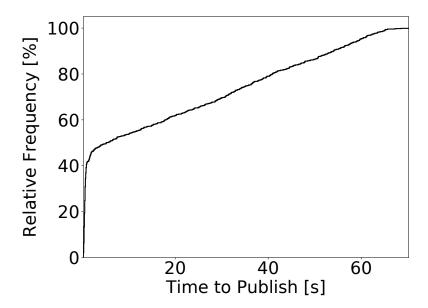
Figure 6.8: Time to content publishing at network partitioning.
