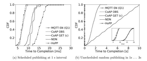
Figure 3.3: Time to content arrival in a single-hop topology.
