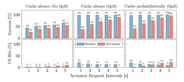
Figure 5.14: Average success rates and cache hits for different levels of actuator request intervals.
