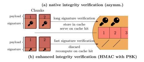
Figure 8.9: Enhanced chunk-wise integrity verification to save device and network resources compared a native NDN protection with asymmetric cryptography.
