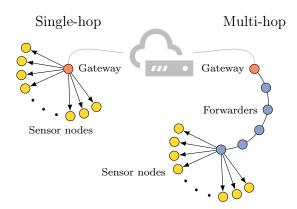
Figure 9.8: Topologies for single-hop and multi-hop experiments.
