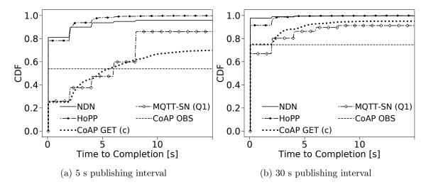
Figure 3.4: Time to content arrival in multi-hop topologies of 50 nodes for publish-subscribe and request-response protocols at different publishing intervals.
