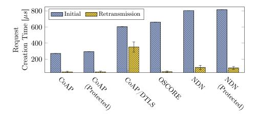
Figure 9.11: Creation time for initial and retransmitted requests.
