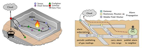
(a) Resilient machine-to-machine communication (b) IoT use cases in industrial settings with device for the Industrial IoT with heterogeneous conmobility and network partitionings. strained IoT devices.
