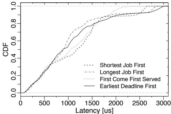
Figure 4: Cumulative Distribution Function (CDF) of End-to-end Latency scheduled with different scheduling algorithms
