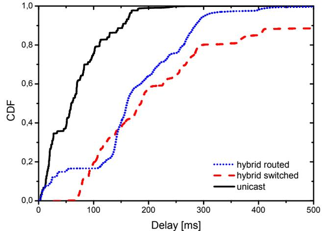
Fig. 5. End-to-end one-way delay distribution for unicast and both hybrid multicast scenarios (switched, routed).
