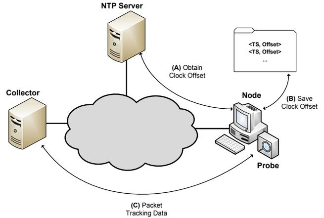
Fig. 1. Time Measurement Setup
