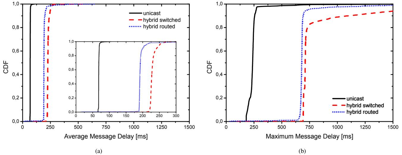
Fig. 6. Comparison of average and maximum one-way packet delay for unicast and both hybrid multicast schemes.
