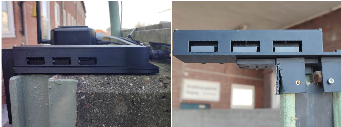
Figure 11: Side view of the mounted housings. The sensor housing mounted on the frame (left). The housing of the magnets on the gate (right).
