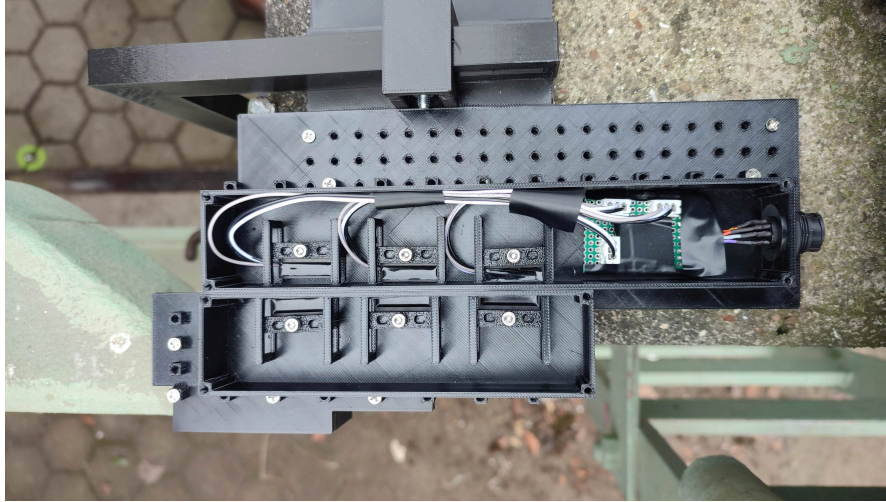
Figure 12: Top view of the mounted housings for the sensors and the magnets without the lid and with the gate closed.
