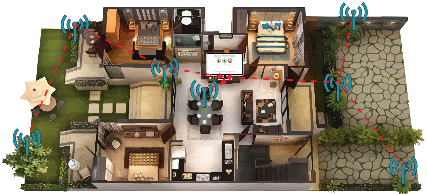
Figure 1. An example of a Watr.li network. The blue antennas depict Plant Nodes and the monitor in the center is the Display Node. The connections between the nodes shows a possible tree topology formed towards the Display Node acting as root node.
