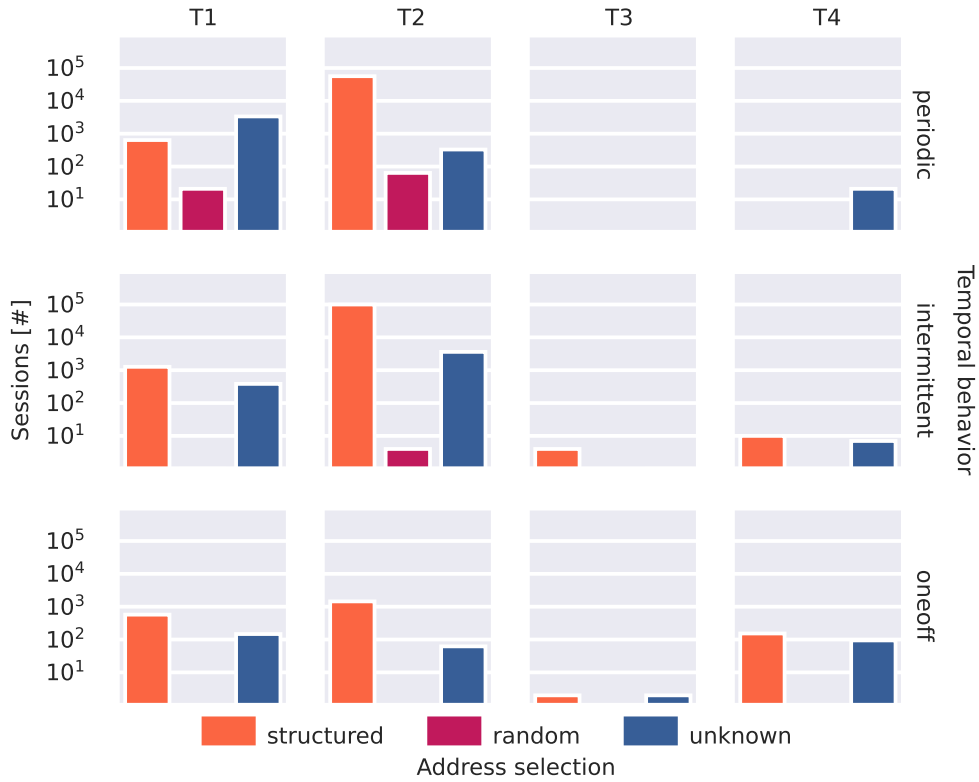
Figure 7.7: Classification of scanners per telescope based on temporal behavior, with a further subdivision of sessions per classification according to address selection, before the split period.
