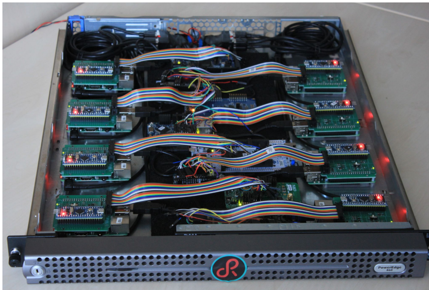
Figure 7.3: A single rack from the HiL testbed of the RIOT community
