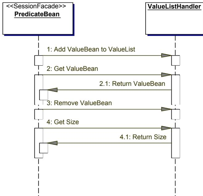
Figure 12: Value List Handler Sequence Diagram
