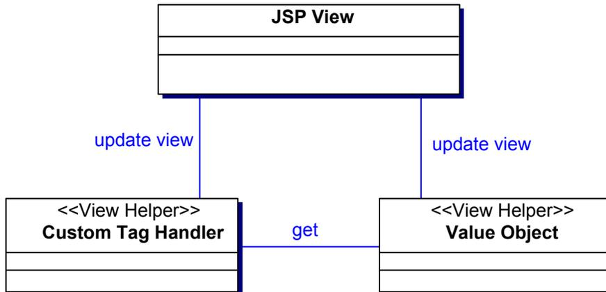
Figure 20: The View Layer Components
